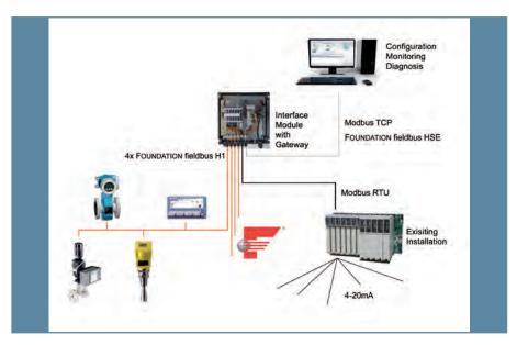
Figure 2: A gateway allows the renewal and expansion of legacy plants by FF components
