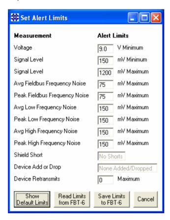
Type in the desired limits for each parameter and click **Save Limits to FBT-6** to write the limits to the PA Monitor.
