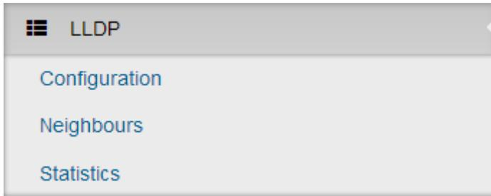
The Link Layer Discovery Protocol (LLDP) is a link layer protocol in the Internet Protocol Suite used by switches to propaganda their identity, capabilities, and neighbors on wired Ethernet network. The protocol is formally referred to by the IEEE as Station and Media Access Control Connectivity Discovery specified in IEEE 802.1AB and IEEE 802.3-2012 section 6 clause 79.
