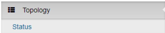
This function gives user a graphical overview of the entire network topology. However, the LLDP function of all the connected switches must be activated to work this out.
