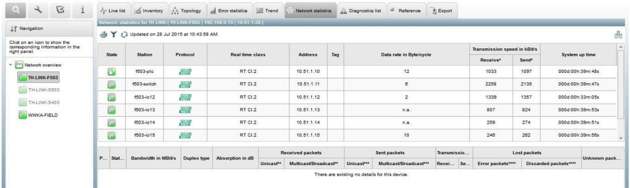
For each station the following information is displayed: state of the station, protocol, address, tag, data rate (incoming and outgoing), network statistics.
