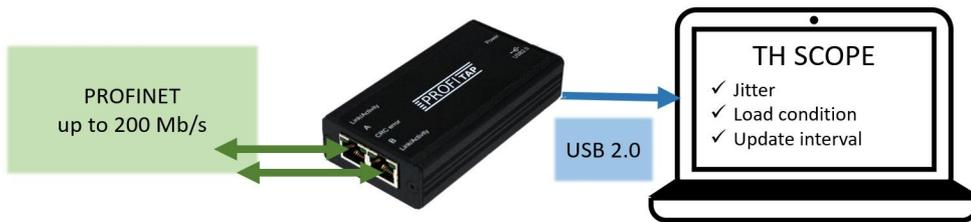
This setup ensures that the frame traffic of each PROFINET device in the network is recorded. What follows is an analysis of the traffic time of the data frames. The measured jitter, load ratio and update intervals are recorded in the acceptance reports.
