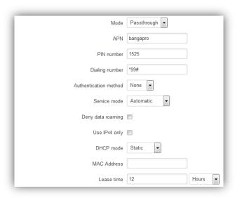
Using Passthrough Mode will disable most of the router capabilities!
