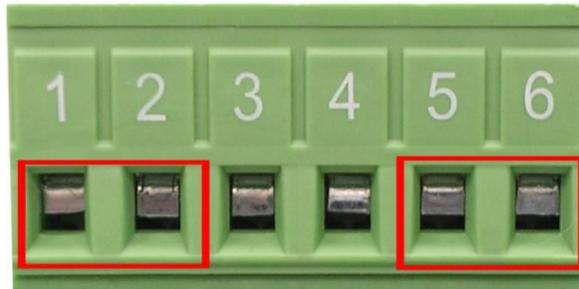
1. Insert AC or DC power wires into the contacts 1 and 2 for power 1, or 5 and 6 for power.
