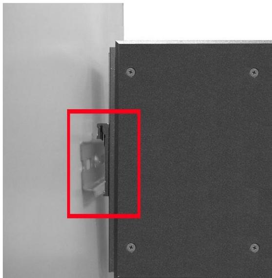
3. Check if the DIN-Rail is tightened on the track or not.
