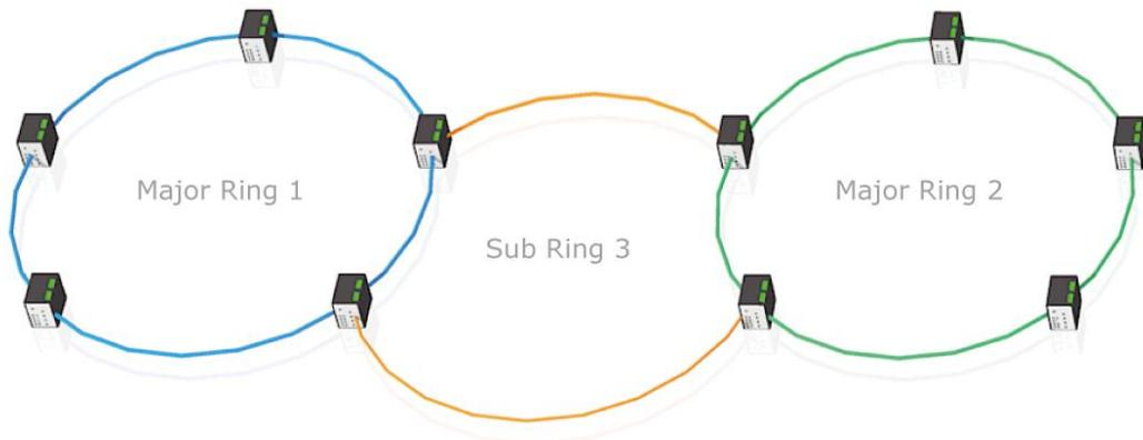
Redundant Coupling with Multiple Rings
