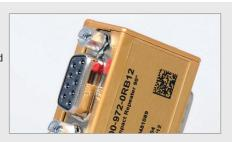
The PROFIBUS Compact Repeater is plugged directly onto the Sub-D socket of the PROFIBUS participant instead of the normal PROFIBUS device connector. It is fastened using the two screws above and underneath the socket.
